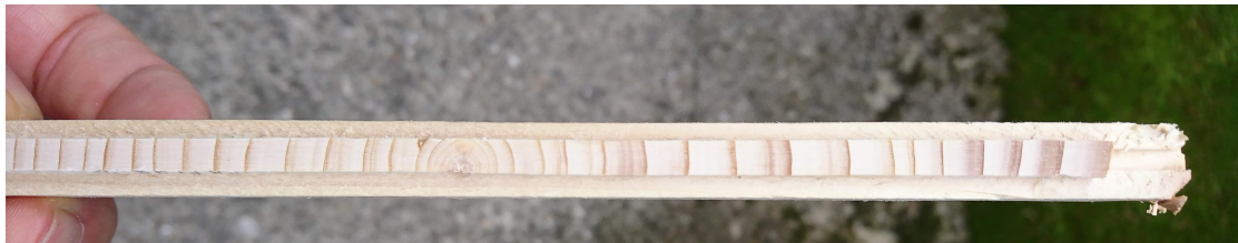
Figure 1.2. A core sample of European oak ( Quercus robur ) with annual rings and pith clearly visible. Taken in September 2018 at the 29 th European Dendroecological Field Week.
